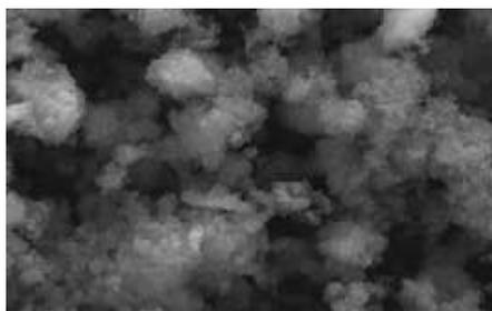
**Fig. 6.** FE-SEM of Iron oxide nanoparticles
