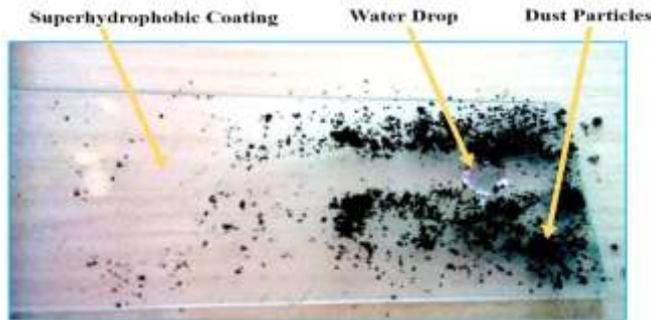
**Fig.3:** Super hydrophobic coating shows Self-cleaning property.
