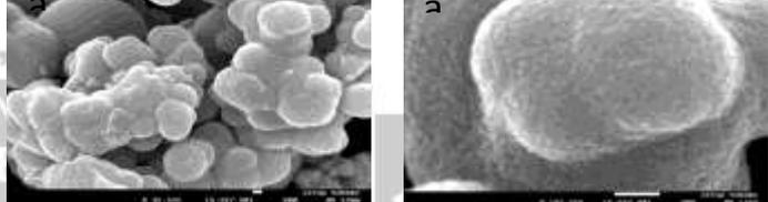
Fig.2: SEM images of SnO<sub>2</sub> with two different magnifications (a1) and (a2).
