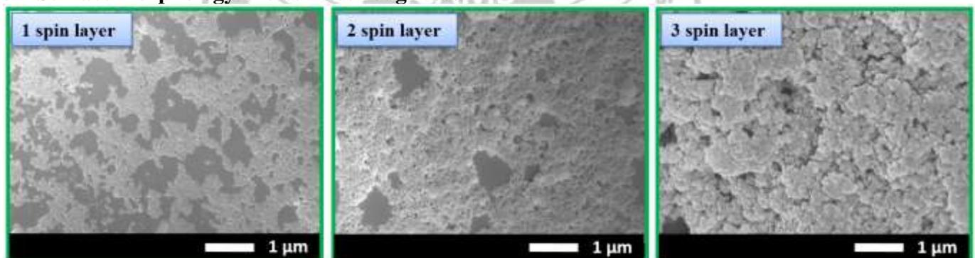
**Fig. 1:** FE-SEM images of SAC samples prepared by 1, 2 and 3 spin deposition layers.
