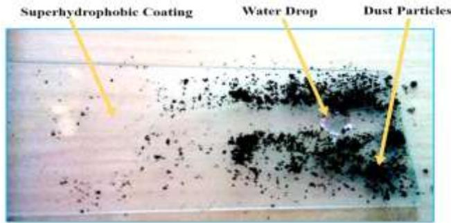
**Fig.3:** Super hydrophobic coating shows Self-cleaning property.
