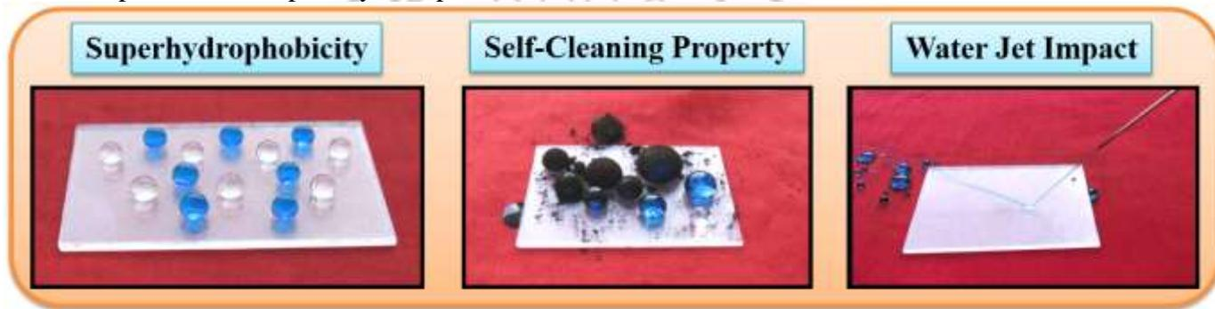
**Fig. 3:** Spherical water drops, self-cleaning property and water jet impact test on 3 spin layer deposited SAC sample.
