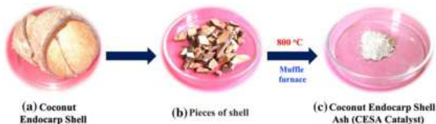
Fig. 2 Preparation of CESA catalyst
